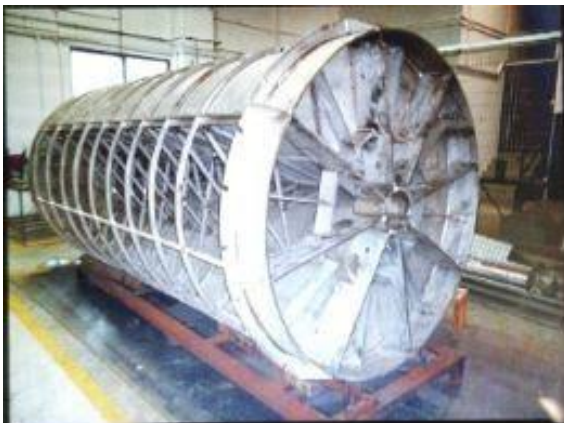
Fabrication of Strainer
